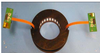
Figure 1: Depicts a 24 – single wrist PET detector ring. The ring has an inner diameter of 100.8 mm and an axial length of 18.3 mm.
