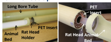
Figure 2: Self containment concept A- Positioning tube with animal bed and transport system B- Shows how the animal head is precisely positioned into the PET/MRI coil array assembly.
